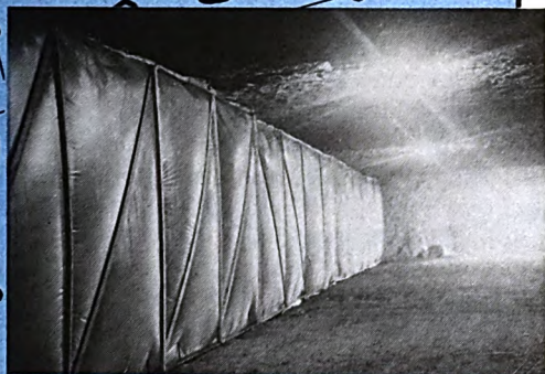
A dividing wall formed by covering wooden frames with polyethylene sheets separated the two adjoining entrances and formed two major areas of mine space. With this arrangement, ventilating air was expelled by the exhaust fans through the mine entrance on one side of the divider wall while fresh air was drawn in through the other entrance on the opposite side of the wall. The fresh incoming air had to traverse one half of the mine space before founding the end of the wall on its way to being expelled as exhaust air.
